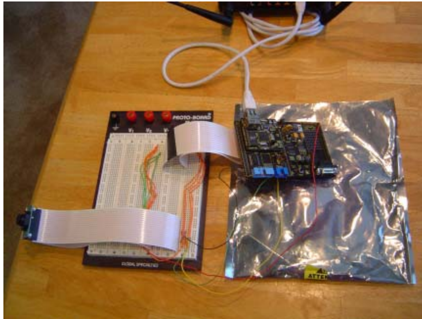
Figure 8. EZ80F91 to breadboard wiring
