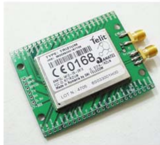
Figure A.2: Spark Fun Electronic's Trizium Evaluation Board
