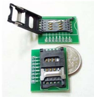
Figure A.4: SIM card Breakout Board
