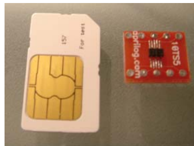
Figure B.4: SIM card and SMT Breadboard adapter with XN04312
