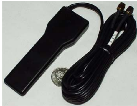
Figure A.6: Covert GPS and GSM antenna
