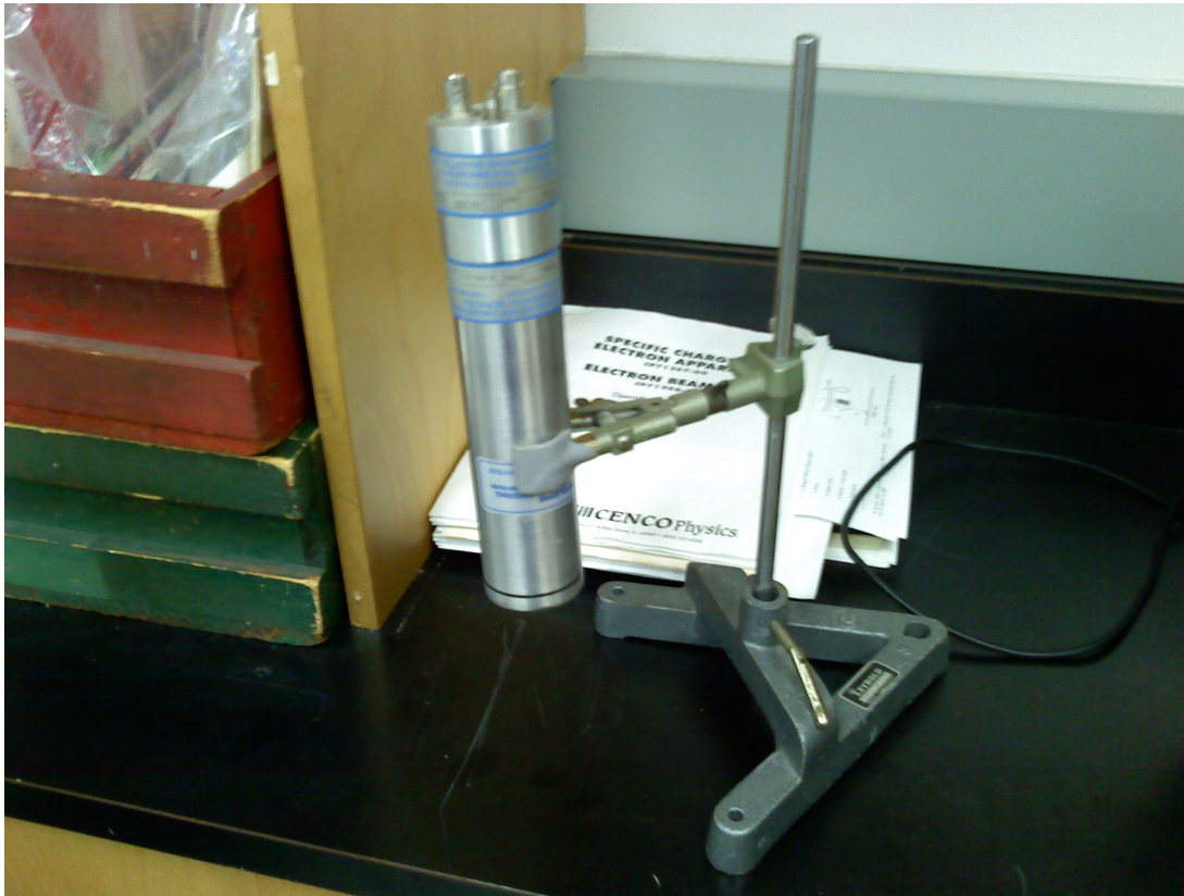
Figure 4.2: NaI(Tl) detector and stand
